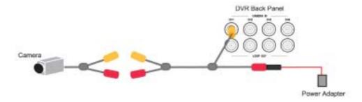
**Connection Type 2** – For cameras that have a VIDEO OUTPUT terminal on the rear panel of the camera body.
